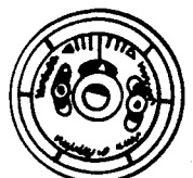
4. Loosen screws, adjust pointer, tighten screws, replace dial.
